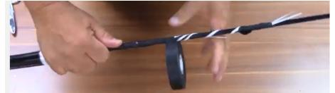
5. Push Grip onto the full length of the exposed Central Member and then tighten the grip.
