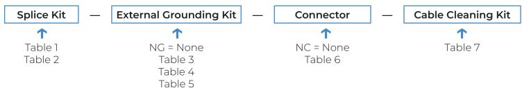
**EXAMPLE:** A request for a 25kV IP Compact Elaspeed Splice Kit with a single #2 AWG Ground Braid, spliced together with 1/0-500 Shear Bolt Connector and Cable Cleaning Kit would be: 25IPES3-GB1200-ALSB3-IP
