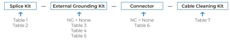
**EXAMPLE:** A request for a 25kV IP Compact Elaspeed Splice Kit with a single #2 AWG Ground Braid, spliced together with 1/0-500 Shear Bolt Connector and Cable Cleaning Kit would be: 25SIPJCeC-GB1200-ALSB3-1P
