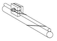
Figure 6 - Lashing Wire Clamp
