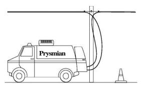
from strand level to a splicing vehicle below plus 16 feet or so of extra slack.
