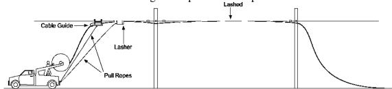
2.01 Two basic methods of lashing fiber optic cable are presented in this document:
