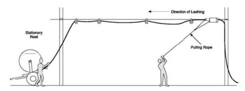
Figure 10 - Pull-back Lashing of Cable
