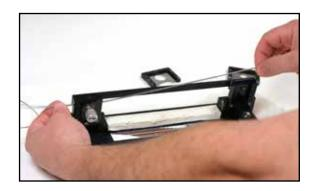
**1.9** Snip the excess fiber ends that are not ribbonized in preparation for splicing.
