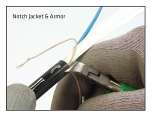
Wrap one ripcord through and around the needle nose pliers. With one hand holding the cable right at the ring cut (B), use the other hand pull the ripcord with the pliers. Pull the ripcord all the way to the end of the access window just beyond ring cut (A). Repeat this step for the second ripcord.
