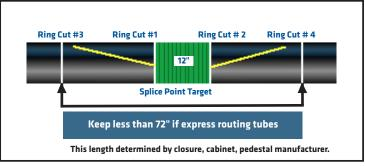
**NOTE:** The switchback point on a loose tube ribbon cable is approximately 18-24" apart.
