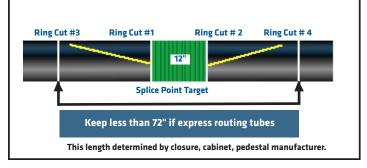
**NOTE:** The switchback point on a loose tube ribbon cable is approximately 16-24 inches apart.
