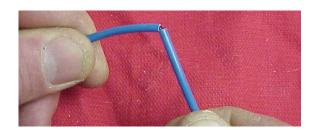
**CAUTION:** Hold the buffer tube tight and straight while pulling the tube off the fibers. Apply back-tension to the fibers while pulling the tube off. It is NOT recommended to push off the tube.
