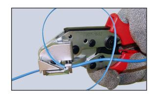
**5.12** Squeeze the handles of the tool together to release the catch and allow the tool to open.
