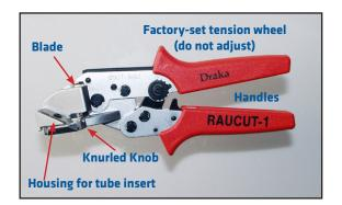
**5.5** Confirm the compatibility of the outside diameter of the tube and the insert. The top of the buffer tube should be approximately flush with the top of the insert, but should not protrude past the top of it.
