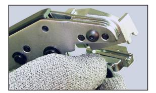
**CAUTION:** Ensure the tube remains in the insert's groove as you close the tool, or the tube can be in advertently crushed.
