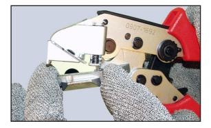
5.7 Turn the knurled knob clockwise to secure the insert.
