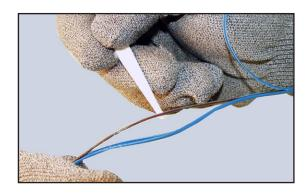
**NOTE:** Cleaning the fibers using this two-step method will provide the best results.
