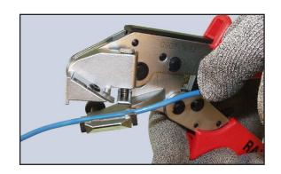
5.11 Hold the buffer tube firmly with one hand. With the other hand, pull the tool along the tube until the desired length of tube has been opened.
