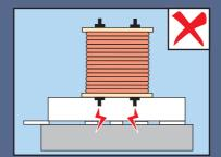
Never lay drums on their side, even on top of pallets, as protruding bolts damage spools and cable.
