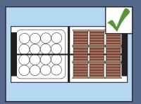
Always protect product, especially spools, against rope damage during tying down of load.
