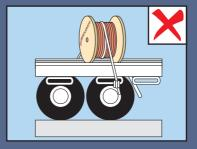
When securing drums for transit, do not place ropes or chains over cable as damage can occur to the outer insulation rendering the cable unserviceable.
