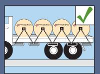
Heavy drums should be chained appropriately for transit, with protection from the chain rubbers for the spindle hole in the centre of the drum. Under no circumstances are drums to be transported on their side.
