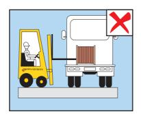
Do not use the fork lift tynes to push cable drums sideways on a truck tray or the ground as damage to the flanges can result in the drum being unacceptable to customers.
