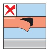
Do not attempt to lift drums of cable without inserting the fork lift tynes fully under both flanges as the tynes can damage the cable, making it unserviceable. Do not attempt to lift drums by the flange or to lift drums into the upright (correct) position by lifting the top flanges as it may break the flange from the drum barrel. The drum will then be undeliverable. Use a length of steel pipe through the centre of the drum to provide leverage and control.
