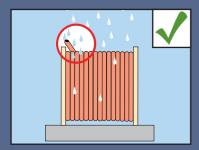
Ensure cable sealing is intact so moisture cannot seep into cable.
