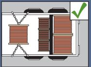
Always protect cable from rubbing or damage. Adjust load or use separators.
