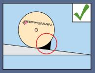
When placing drums on an uneven surface be prepared to check drums against rolling and chock if required.
