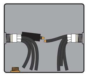
Install compression connector over exposed conductor ends and crimp with correct color-coded die.
