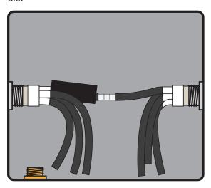
i) Cut strip of Lifeline® Ceramifiable tape and wrap connector at 45-degree angle with 50 percent overlap. Start wrapping over insulation with leading edge of tape aligned with one side of connector, continue wrapping until other side of connector is reached, and connector is covered by tape two layers thick.
