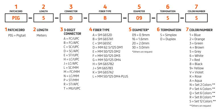
The pigtail color code can be seen in the table below. When ordering sets of pigtails, they are supplied with the colors from 1 to 12. For example if a set of 6 pigtails is ordered the colors supplied are Blue, Orange, Green, Brown, Grey, White.
