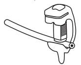
Removal of outer sheath can be done with a special circle cutting tool or with an ordinary knife since the layer under the sheath is steel wire braiding. This braiding will protect the cable core
