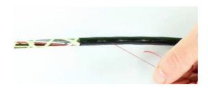
**5.13** Ring the jacket again and remove the excess sheath. Use your snips or other approved tool to remove the yarns, water blocking material, and rip cord.
