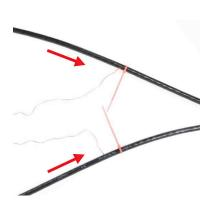
**6.16** Use your calibrated tool to ring the jacket at each mark on the cable.
