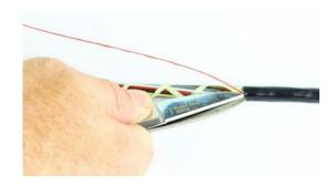
**5.12** Pull the rip cord out of the jacket for the desired length of cable that you wish to open.
