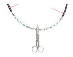
**6.14** Use your snips to notch the jacket to allow the rip cord to pull easily.
