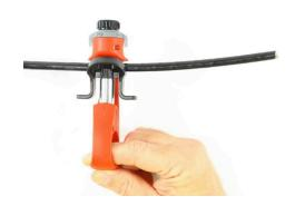
**5.8 DO NOT REMOVE THE TOOL FROM THE CABLE.** Switch the tool to Longitudinal cut.
