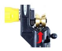
**6.5** Here the blade has been adjusted to the proper depth. This will score the sheath with out damaging the underlying tubes.
