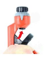
**5.4** Use a scrap piece of cable to guage the proper depth. This is too deep. The blade extends too far into the jacket and will cut the tubes.
