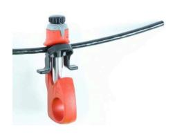
**5.9** Gripping the tool firmly, slide the tool off the end of the cable.
