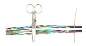
**6.20** Use Vinyl tape to secure the ends of the cable from fraying or chaffing.
