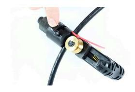
**6.10** Shift your blade to longitudinal cut and pull the tool to the next mark across the apex.
