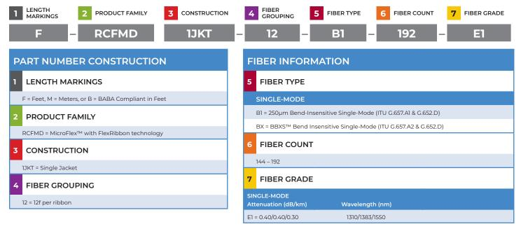
**Notes:** Please refer to the Fiber Code Addendum for additional fiber options, or contact us for help. For individual fiber breakout, please refer to Prysmian's FlexRibbon breakout procedure.
